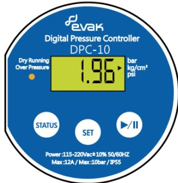
2). Min. Start pressure setting (low pressure) (Show code P-min)
